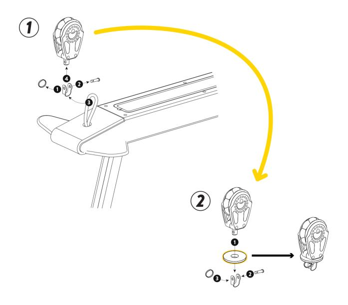
(1) Remove the split ring from your ratchet pulley to detach it from the lanyard.
