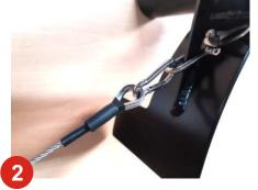
When assembling the boat, attach the wires with the straining devices as shown on the photo.
