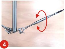
When the boat is assembled, tighten the straining devices so that the wires are strongly stretched.
